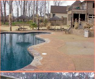
This is a beautiful mix of hardscape materials! The pool coping is natural stone. The deck is a combination of stamped concrete and washed/exposed aggregate concrete. The retaining/seating walls in the background are old brick. A gorgeous combination!
